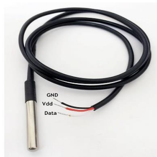
Fig- 5: Temperature sensor
